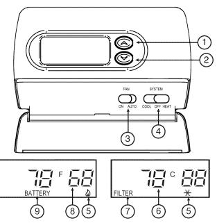
Figure 8. Thermostat display, buttons, and switches
